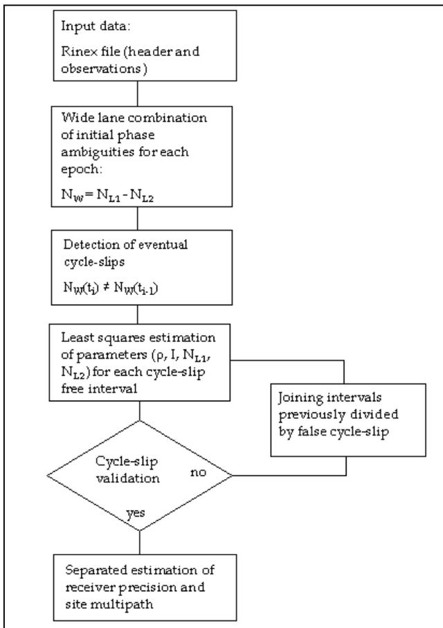
Fig.1 - Flow chart of PERMGPS-QC software
