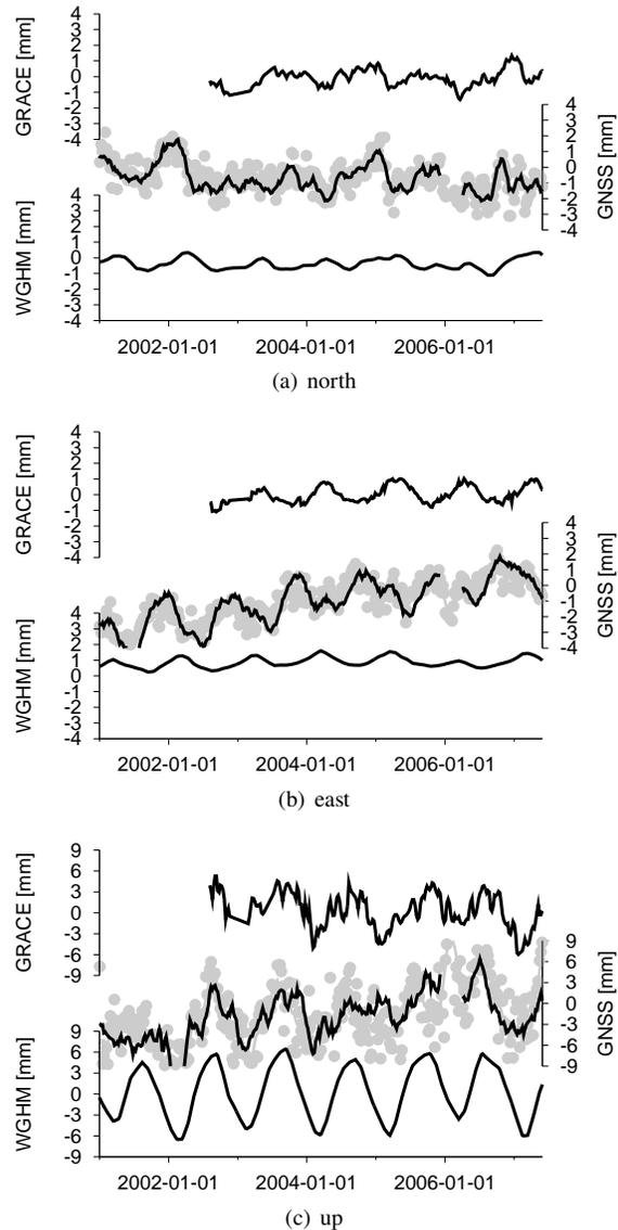
**Fig. 2.** North, east and vertical component of GNSS solution (from IGS, gray dots) and smoothed time series (gray line, see text) along with modelled deformation from GRACE and WGHM for Lamkówo site (LAMA). The black solid line indicate smooth GNSS solution with ATML subtracted. Note different scale for horizontal and vertical components.
